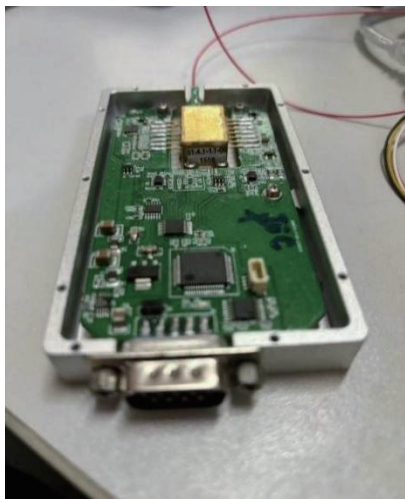
(a) F-P微外腔自注入锁定窄线宽激光器模块 (a) F-P external cavity self-injection-locked narrow-linewidth laser module
