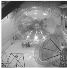
(b) 大口径可折叠展开式薄膜发射望远镜示意图 (b) Large calibre deployable membrane launching telescope configuration
