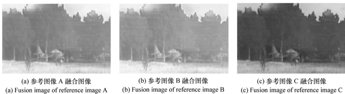
图5 区域能量法彩色融合图像(色彩传递公式中 a = b = 1, m_C = m_{B,C} = m_{R,C} = 0 )
