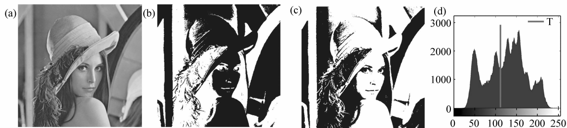
Fig. 2 (a) Original image of Lena. (b), (c) Separation results using the single threshold Otsu's method. (d) Location of threshold using the single threshold Otsu's method
