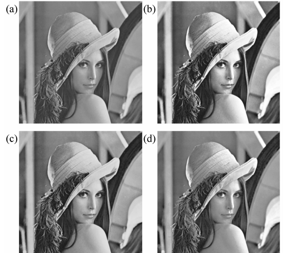
Fig. 5 (a) Original image of Lena. (b) Result of GHE. (c) Result of RLBHE. (d) Result of RLAMHE
