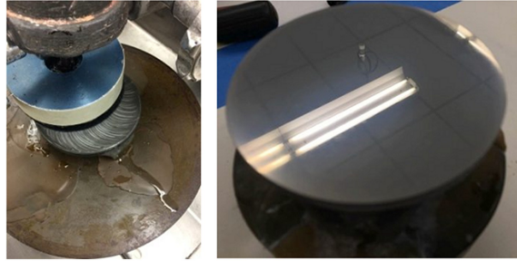
(a) 反射镜抛光 (a) Mirror polishing (b) 抛光后的反射镜 (b) Mirror after polishing
