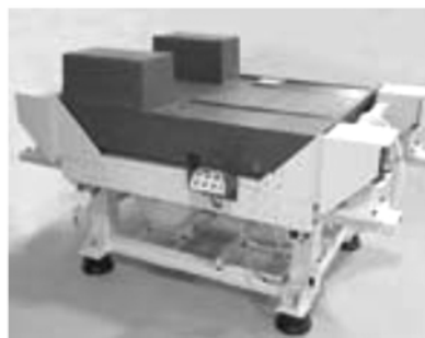
图7 Nanoform 700 ultra的床身与隔振系统 Fig.7 Base and vibration isolation system of Nanoform 700 ultra
