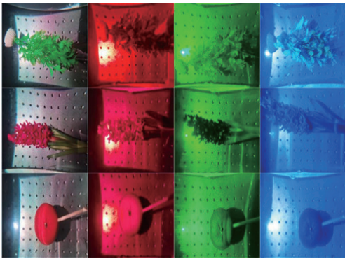
Fig. 9 The lighting effect of different light sources illuminating green leaves, safflower and orange targets in clear water at a distance of 19 cm from the water surface
