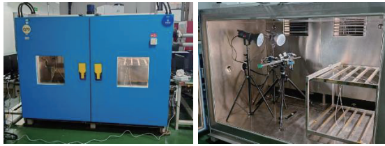
(a) 温湿度环境箱 (b) 测试装置 (a) Temperature-humidity chamber (b) Testing equipment
