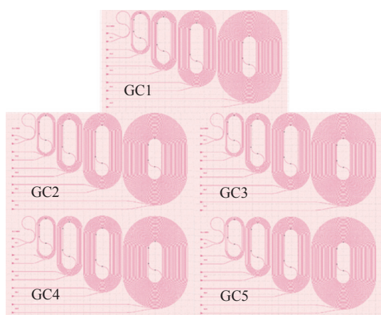
Fig. 4 Layout image of the 5 sets of cutback structures for the 5 splits of the grating coupler
